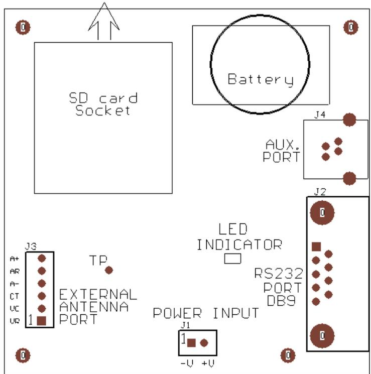
Fig 2. Main Unit connector diagram.
