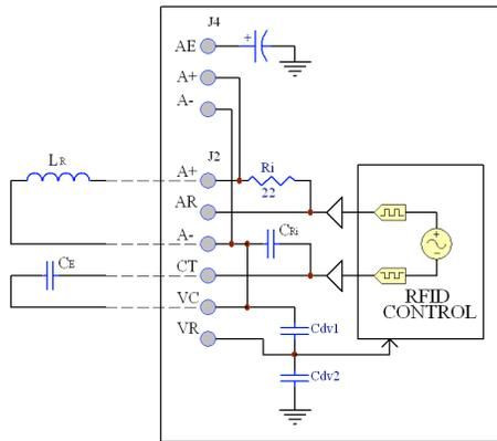
Figure 2. Antenna Drive Interface
