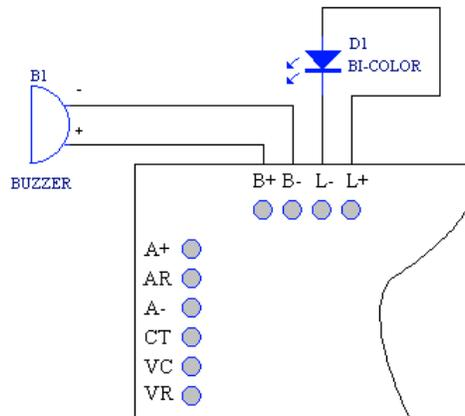
The L+ output line has a 1K ohm current limit resistor placed in series located on the RFID485 unit. The maximum current drive available for the Buzzer output B- line is 100mA.
